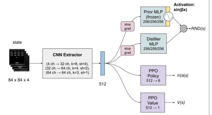
Architecture for parallel training of PPO (purple) and RND (green), which itself consists of a frozen prior network and learned distiller. A feature extractor learned under PPO is also used as a feature extractor for the RND networks, but does not receive weight updates from the RND.
